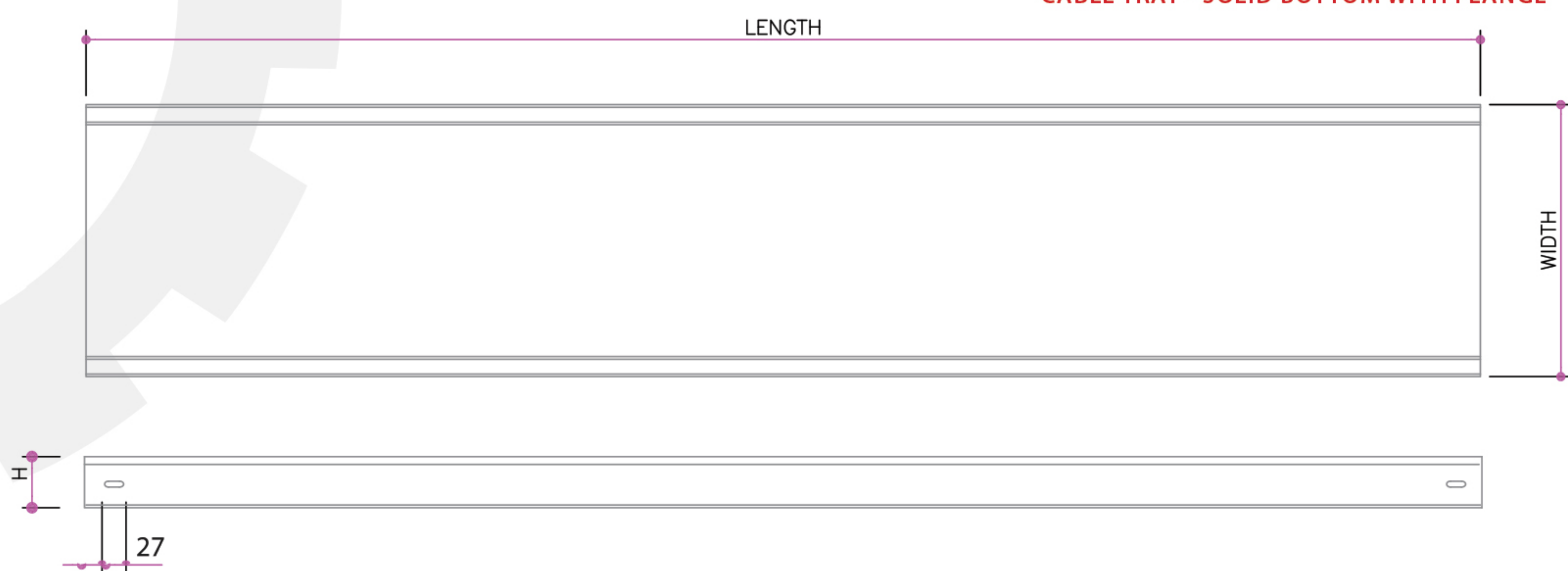
CABLE TRAY - SOLID BOTTOM WITH FLANGE
